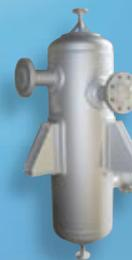
Stainless steel pulsation dampers for methane gas, operating at 42 bar(g) with temperatures ranging from  $-150^{\circ}\text{C}$  to  $+170^{\circ}\text{C}$ , and featuring U-stamp and AS1210 (Australia) approvals.
