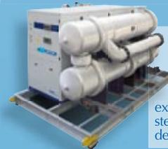
Dryer operating with chilled water for 4 bar(g) operation in the glass industry, featuring cooling and air-to-air exchangers with stainless steel tubes and a double demister separator.
